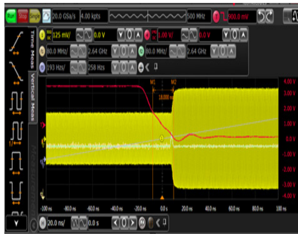
Figure 22. Power ON Switching Time
