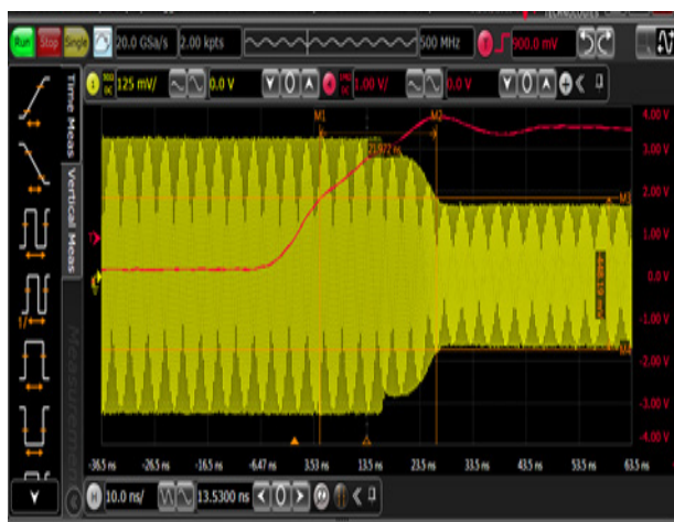
Figure 21. Power OFF Switching Time
