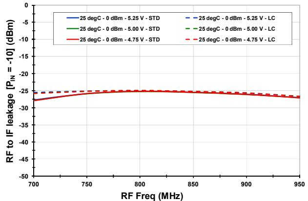
**RF-IF Leakage vs. LO Level**
