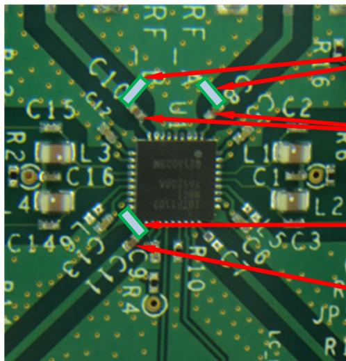
Scrape resist from ground and add shunt 8 pF
