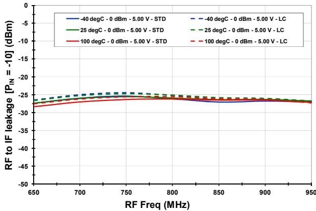
**RF-IF Leakage vs.  $V_{CC}$**
