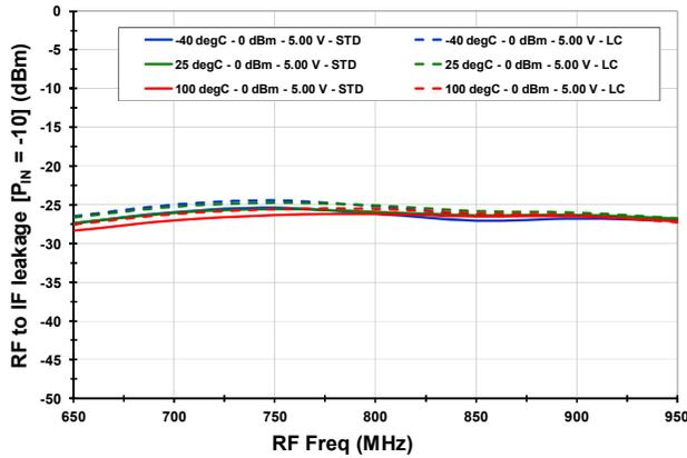
**RF-IF Leakage vs. V<sub>CC</sub>**
