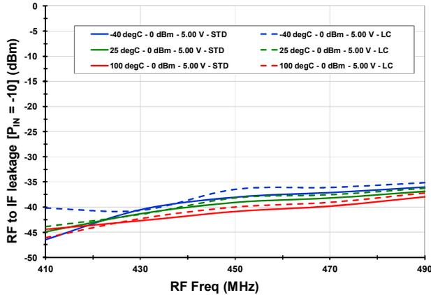
RF to IF Leakage vs. LO Level (130 MHz IF)
