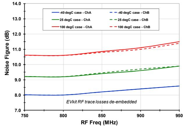
Noise Figure vs. T<sub>CASE</sub> (STD Mode)
