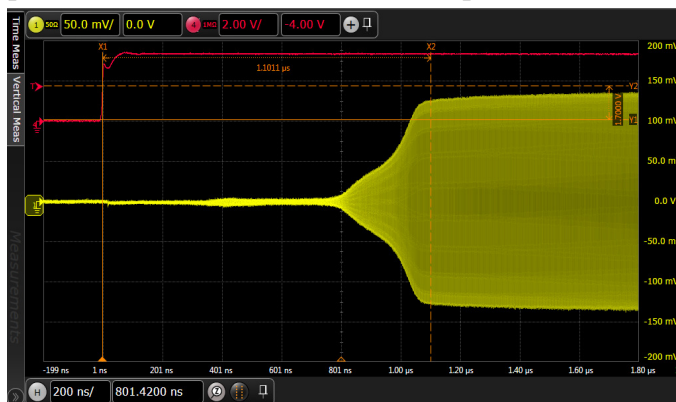
Figure 24. Switching Time [Isolation to Insertion Loss State]
