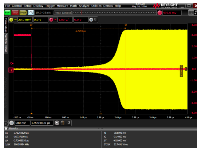
Figure 19. Switching Time Isolation to Insertion Loss
