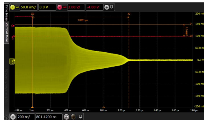
Figure 15. Switching Time [Insertion Loss to Isolation State]
