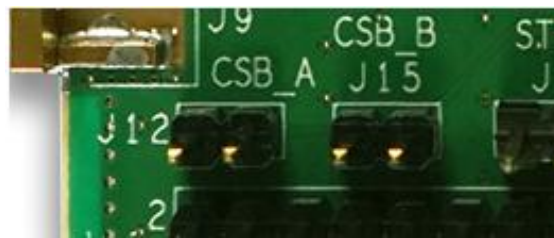
Figure 80. Jumpers for Serial Programming Connections
