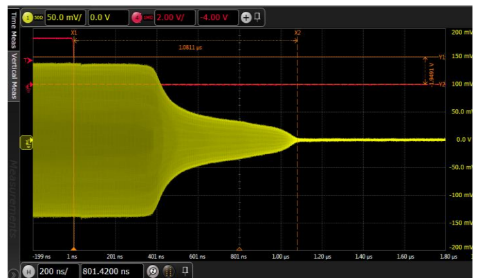
Figure 25. Switching Time [Insertion Loss to Isolation State]
