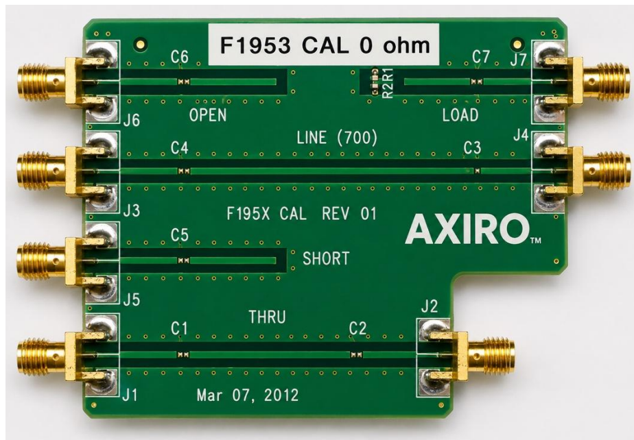
Standards used for F195x TRL calibration
