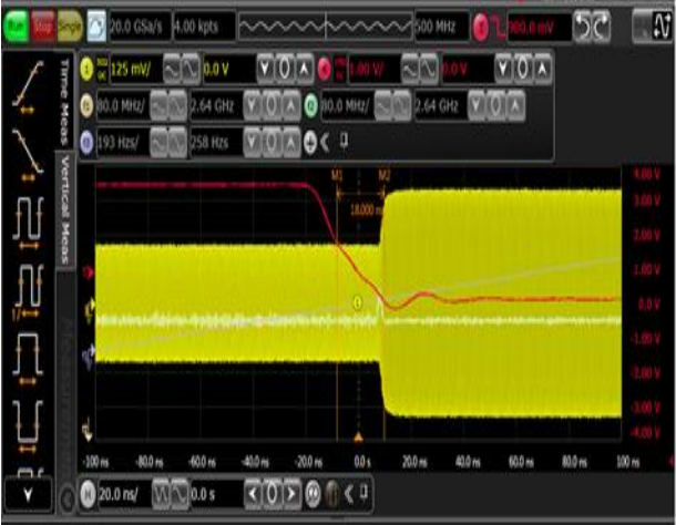
Figure 22. Power ON Switching Time
