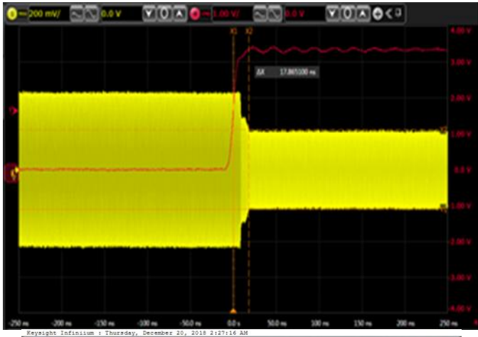
Figure 19. Gain Settling Time
