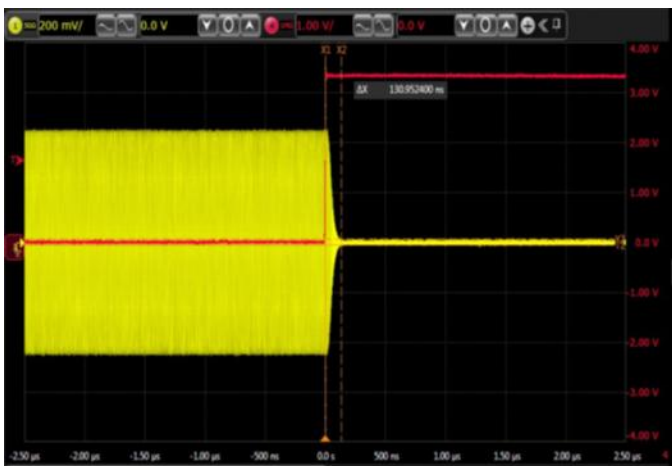
Figure 23. Power OFF to Standby Mode
