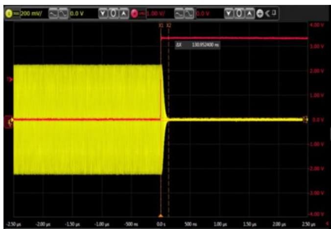
Figure 23. Power OFF to Standby Mode
