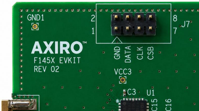
Figure 53. Image of J7 Connector for SPI
