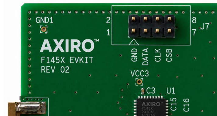
Figure 69. J7 Connector for SPI
