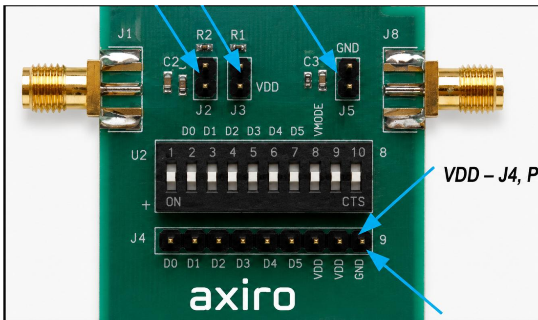
Figure 24. Power Supply and Logic Voltage Connections
